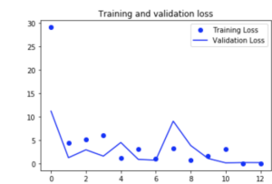
Fig. 25. Loss of the Model Trained Without Augmenting the Training Set
