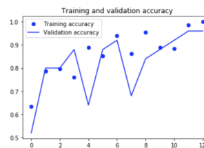
Fig. 24. Accuracy of the Model Trained Without Augmenting the Training Set
