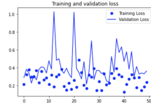
Fig. 40. Loss of the Model Trained With Augmented Training Set (Clean Version)
