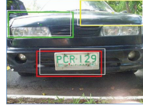
Figure 9: Three hypotheses from coarse localization (red=1st, yellow=2nd, green=3rd) and each of their adjusted boxes (nearest white box).
