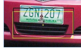
Figure 8: A LP image with the coarse output box (yellow) and the adjusted box (black).
