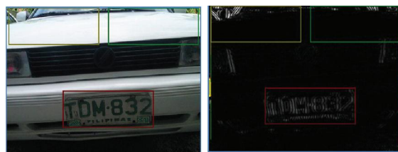
Figure 14: A case where a true positive was eliminated. Notice that the edges in the edge image are weak due to low ambient lighting.
