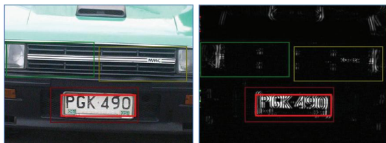
Figure 11: An image containing 3 hypotheses with the coarse (thin boxes) and the resized outputs(thicker boxes). After guess elimination, the only remaining box was the first guess (red).
