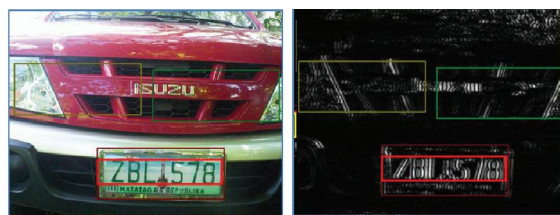
Figure 13: An example of a good resizing. Note that the red bounding box tightly encloses the character row of the license plate.
