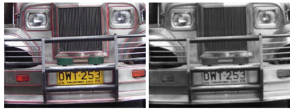
Figure 3: Example of a difficult case (original image and its grayscale). The grills of the jeepney result in high edge content, misleading most edge-based algorithms.
