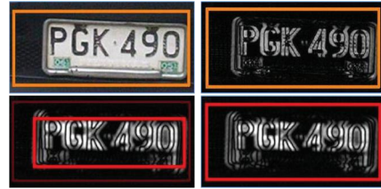
Figure 10: Clockwise from top left: (1) A license plate image, (2) its 1st derivative edges, (3) its 2nd derivative edges, and (4) the new plate hypothesis after resizing the bounding box.
